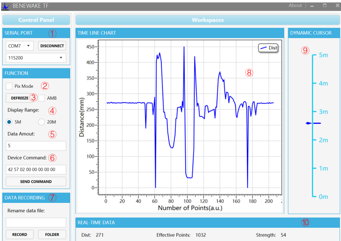
Fig. 5 Client Interface of Distance Measurement Demonstration in Windows
